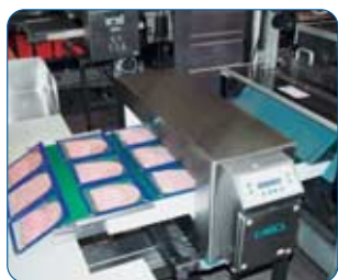
METAL SHARK® BD in line behind a deep drawing machine
