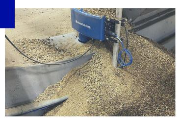
Other technologies require constant re-calibrations, have height interference, experience drifting over time, produce less reflected light energy and overall provide the user with more of an estimated guess of moisture content rather than true, repeatable data. MoistTech's technology provides hundreds of readings per second with the ability to be displayed anywhere throughout the process, giving full access and capabilities to the production line.
