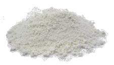
Hydrated lime has multiple uses including building materials, civil engineering, the chemical industry, agriculture, drinking water treatment and sewage treatment. The angle of repose for hydrated lime varies considerably with moisture content. Too much moisture can cause the product to clump, causing blockages in slaked lime and difficulty in loading and transporting material.
