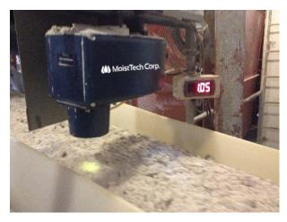
Unlike other instrumentation of this type, some of the unique features of the IR-3000 is that it can monitor the product even with small gaps in product flow and is unaffected by ambient light without impacting the accuracy. The IR-3000 is also ideal for installations on chain conveyors and screw conveyors. The MoistTech IR-3000 gauge is positioned at the exit of the lime shaker, 4-12 inches above the hydrated lime.
