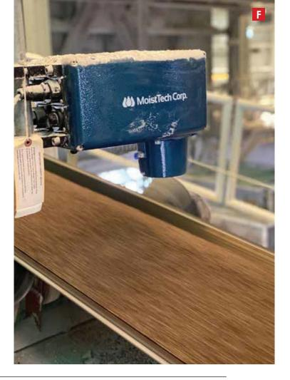
Designed to provide accuracy and repeatability, the MoistTech NIR technology is a ratio-based measurement with prime beam; this eliminates the sensitivity to distance, improves stability and accuracy; whilst the algorithms, wavelengths and sensor optical requirements enable the sensor to take thousands of detailed, accurate measurements per second.
